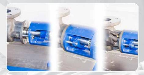
Bolt the Suction Housing to the Bearing Housing with 4x 1/2" bolts with a 3/4" wrench.
