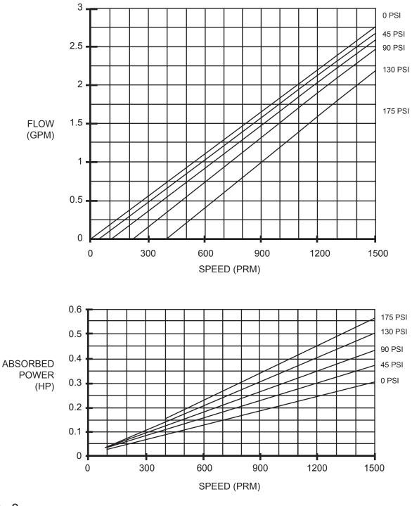
Size: 3 Stage(s): 2 Starting Torque = 3.7 to 4.8 ft. lb Max Pres. = 175 PSI RPM = 0 - 1500
