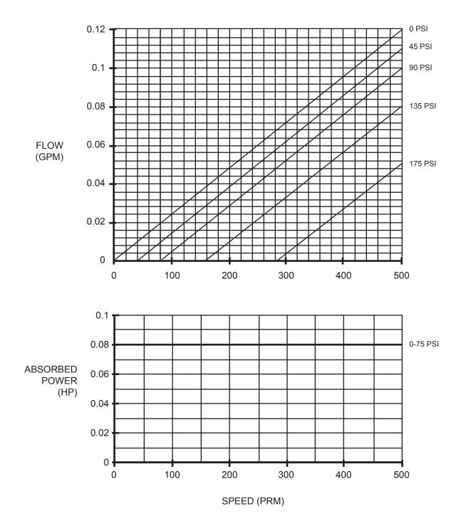
Size: 0.40 Stage(s): 3 Starting Torque = 0.4 to 0.9 ft. lb Max Pres. = 175 PSI RPM = 0 - 500
