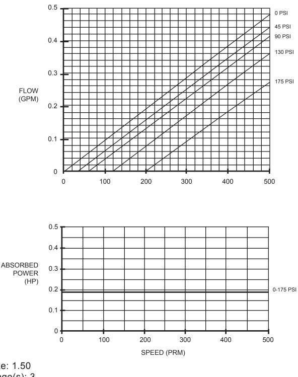
Size: 1.50 Stage(s): 3 Starting Torque = 1.7 to 3.4 ft. lb Max Pres. = 175 PSI RPM = 0 - 500
