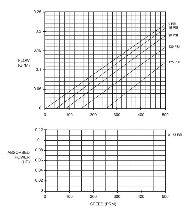
Size: 0.80 Stage(s): 3 Starting Torque = 1.3 to 2.6 ft. lb Max Pres. = 175 PSI RPM = 0 - 500
